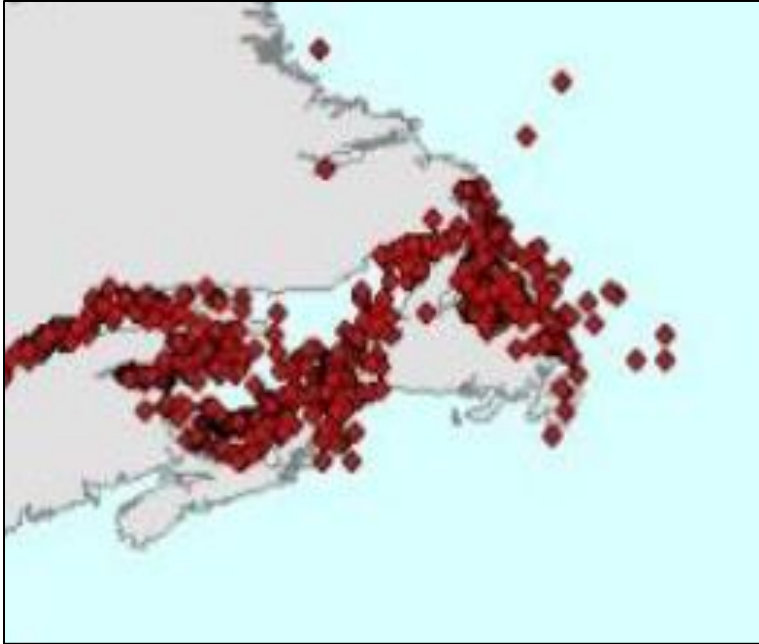
Figure 4. Location of reported incidents of ship besetting and damage due to ice pressure.
