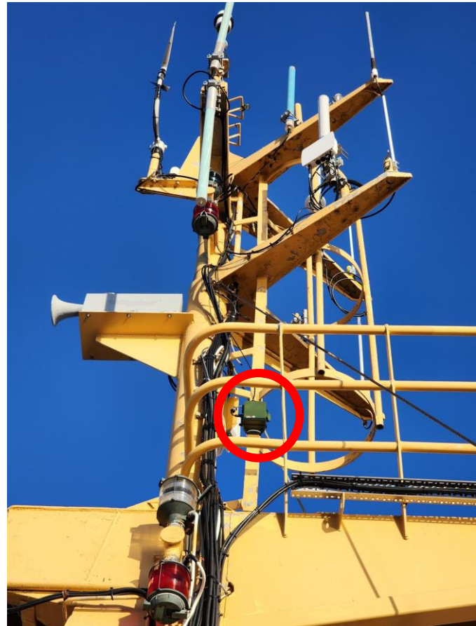
Figure 2: Vessel-mounted Autonomous Recording Unit and Ultrasonic Microphone.
