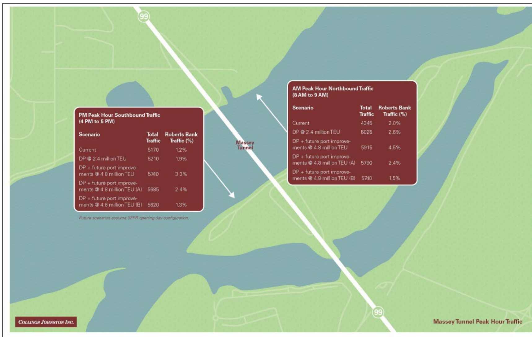
Figure 3 George Massey Tunnel Peak Hour Traffic.
