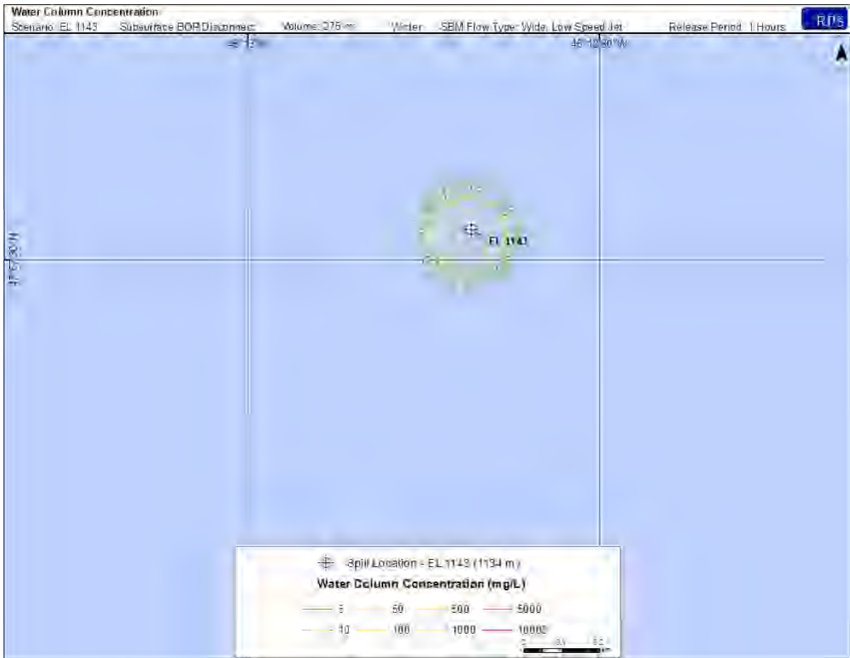
Figure 16-52 Predicted water column concentration from a BOP disconnect accidental seabed release 275 m 3 at Site 1 (Winter)
