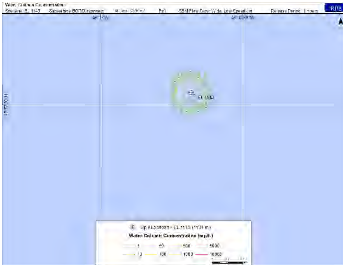
Figure 16-50 Predicted water column concentration from a BOP disconnect accidental seabed release 275 m 3 at Site 1 (Fall)
