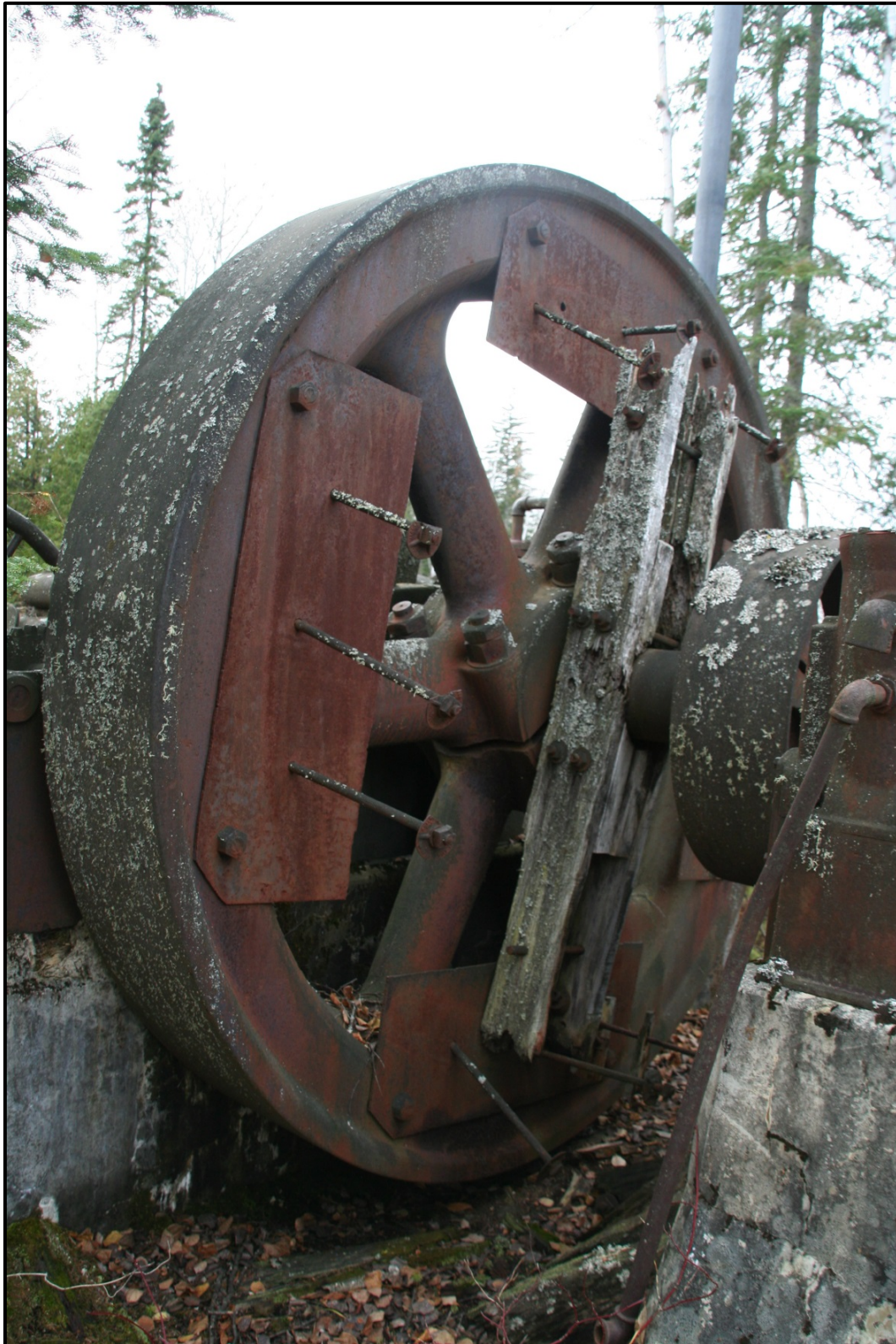
Plate S-16: Keighley Engine, flywheel/belt drive
