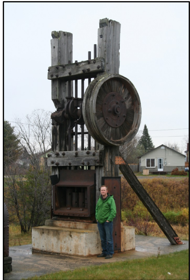
Figure 8: Mining, Stamp Mill (right), originally from the Golden Winner Gold Mine and relocated to park. Atitokan Historical Park Oct 23, 2014
