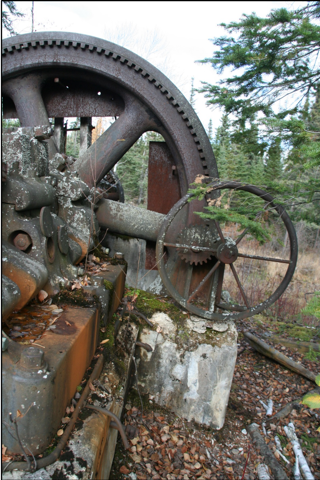
Plate S-15: Keighley Engine, flywheel
