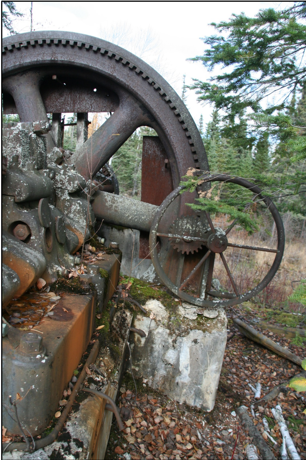
Plate S-15: Keighley Engine, flywheel
