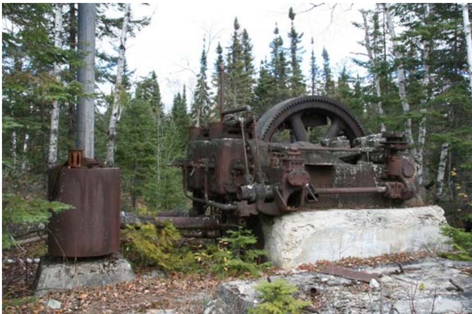
Figure 1: Keighley Engine with exhaust manifold/pipe on left at Sawbill Mine (October 21, 2014)
